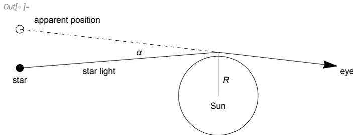
There are five quantities and three independent dimensions. The Buckingham Pi theorem tells us that the solution can be expressed in terms of two dimensionless groups. One group is the bending angle  $\Pi_1 = \alpha$  (it is dimensionless). The other group can be found by inspection. It is  $\Pi_2 = GM / (c^2 R)$ . The formal result of the Pi theorem is
